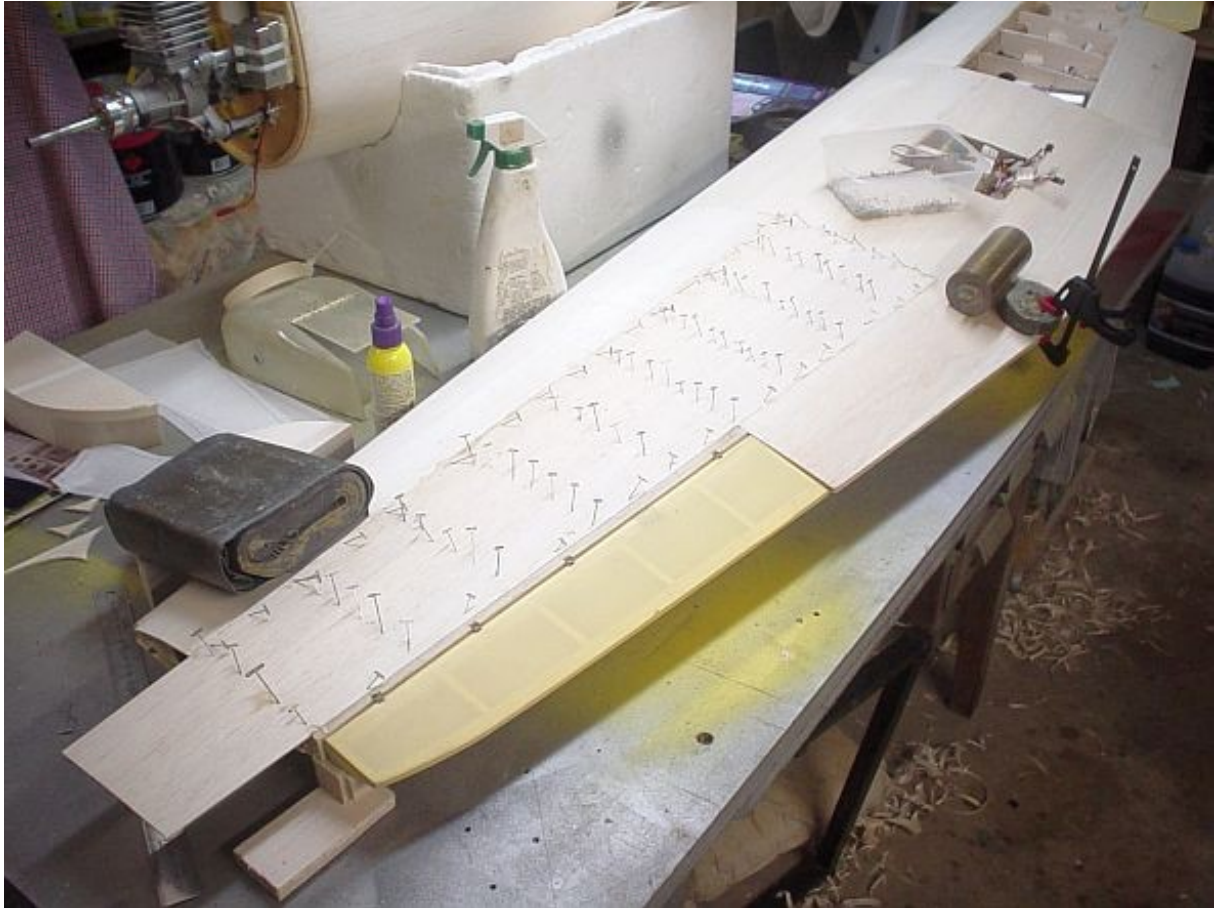
You can see from the above photo that the wing is weighted and clamped to the bench to give the correct twist. It is important to have good glue joins on the skin to the ribs and spars hence the extensive pinning of the sheet to the ribs and spars.
